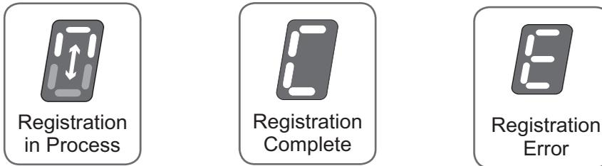
Figure 35: Registration digital displays.
